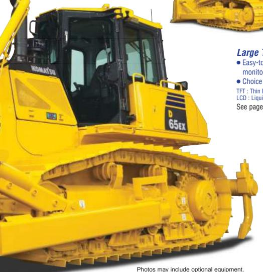
**Modular power train** for increased serviceability and durability. Forward mounted pivot shafts isolate final drives from blade loads. See page 9.
