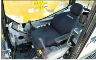
operational posture of armrest together with the console. Reclining the seat further enables you to place it into the fully flat state with the headrest attached.
