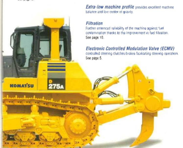
Low-drive, long-track, seven roller undercarriage ensures outstanding grading ability and stability.
