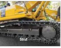
Komatsu PC450LC-7 uses track links with strut providing superb durability.
