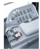
1:Cut-off ON/OFF switch 2:Cut-off adjustment switch 3:Fan reverse ON/OFF switch 4:Boom control 5:Bucket control
