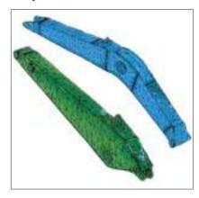
The revolving frame, center frame, undercarriage and attachment structure are designed by using advanced three-dimensional CAD and FEM analysis technology.
