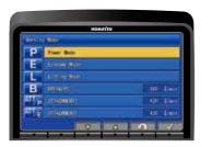
match engine speed and pump output to the application. This provides the flexibility to match equipment performance to the job at hand.
