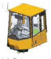
ROPS (ISO 3471): Roll-over Protective Structure FOPS (ISO 3449): Falling Objects Protective Structure
