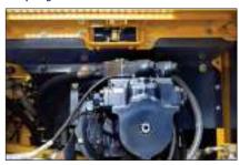
Prevents oil from spraying on the engine if a hydraulic hose bursts.
